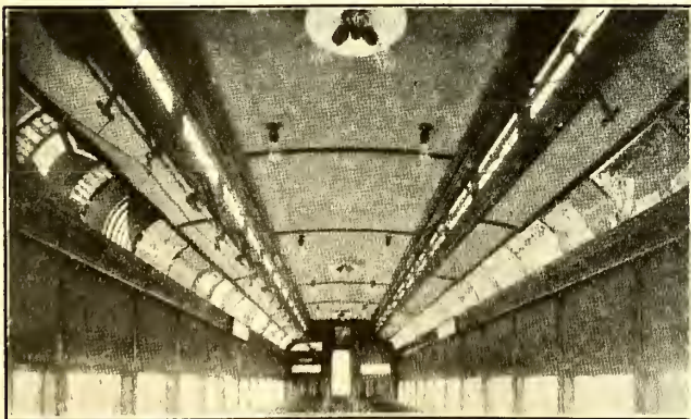
INTERIOR OF CAR SHOWING FORMER ARRANGEMENT OF LAMPS
